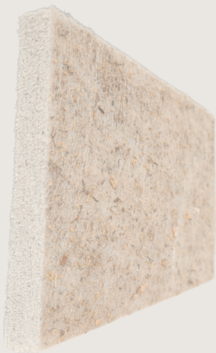
UNPAINTED PEAT-FIBRE SURFACE
