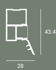
CONSTRUCTION PROFILE WITH DIFFUSER
